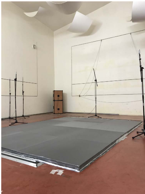
Figure 10. Picture of the measurement set-up in the reverberation room showing the material under test, 5 of the 8 microphones and a group of two sources.
