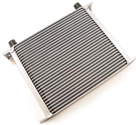
Figure 1: Studied HX - a 30 rows triangular louvered fin aluminum car oil radiator with dimensions L 285mm * l 235mm * h 50mm.
