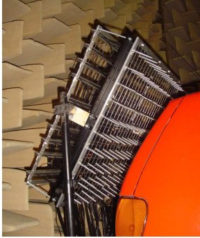
Figure 3 : position of the array for rear wiper noise measurements
