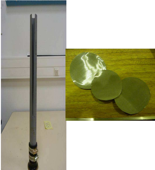
Figure 4 Gradual slit termination and metallic wire mesh
