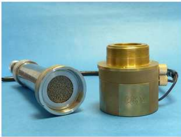
Figure 1 : Impedance Transducer with duct for absorbing materials.
