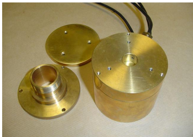
Figure 3: Head of the impedance sensor + adaptor and “infinite impedance load”
