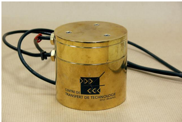
Figure 2: Impedance sensor (including a rigid plate at the input of the impedance head)
