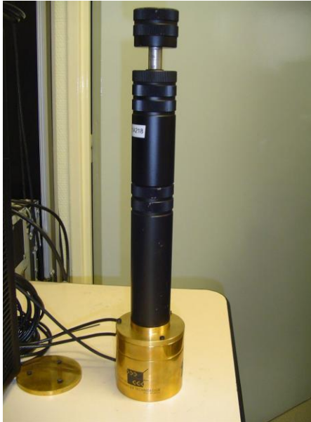
Figure 4: Impedance sensor with 29mm diameter sample holder
