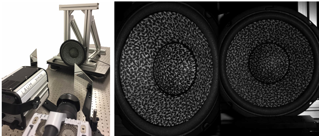
Figure 9. Picture of the experimental set-up. Figure 10. Example of image obtained with the pseudo stereo system with a two-mirror adapter.
