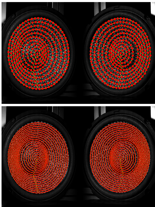
Figure 5. Measurement points re-projected onto the initial images: ( left ) first iteration, ( right ) second iteration.
